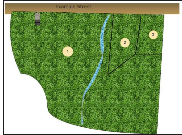
Example 2: Lot Size Averaging Subdivision: A 160-acre parcel subdivided using lot-size-averaging allows the original landowner to retain the vast majority of his/her property, while subdividing the same number of properties as the underlying Forest Conservation District would allow in a conventional subdivision.
